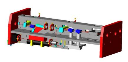
laser has very rigid massive middle and side plates, ensuring a very high stability in the oscillator and pre-amplifier. The dimensions of the laser housing are much smaller than before, making the laser as compact as possible, while still allowing space for two frequency conversion units inside the laser.
