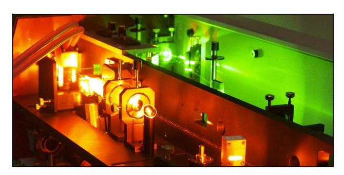
Our NarrowScan series with polarization matched oscillator is ideal for multi-kHz, Q-switched pump sources. The high power dye laser output with high spectral purity and stability can be frequency doubled with high conversion efficiency.
