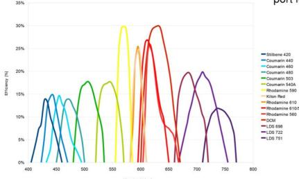
Dye Tuning Curves and Dye Efficiency of the NarrowScan Dye Laser Nd:YAG pumped by 355 nm and 532 nm.
