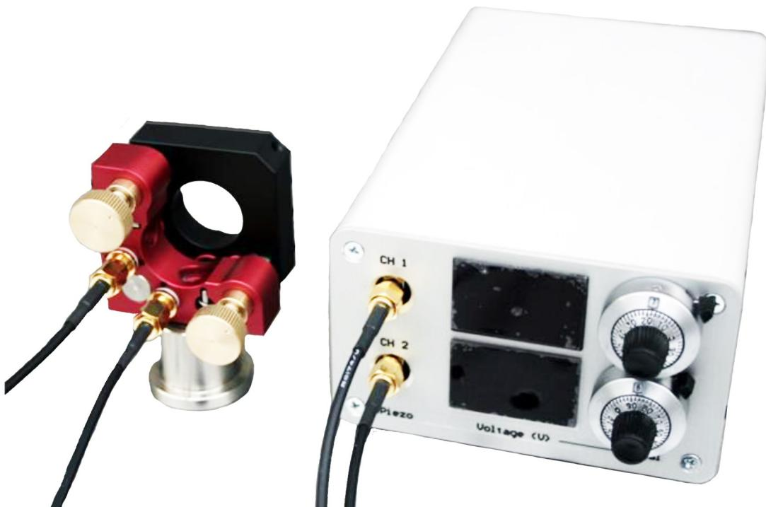
The **MDI-H with Piezo Drive** is a mirror mount which is controlled by a piezo system with our own electronics. Besides a manual adjustment by 0.15 mm / 0.25 mm per turn, the systems can be adjusted electronically within a  $\mu\text{m}$ -range.
